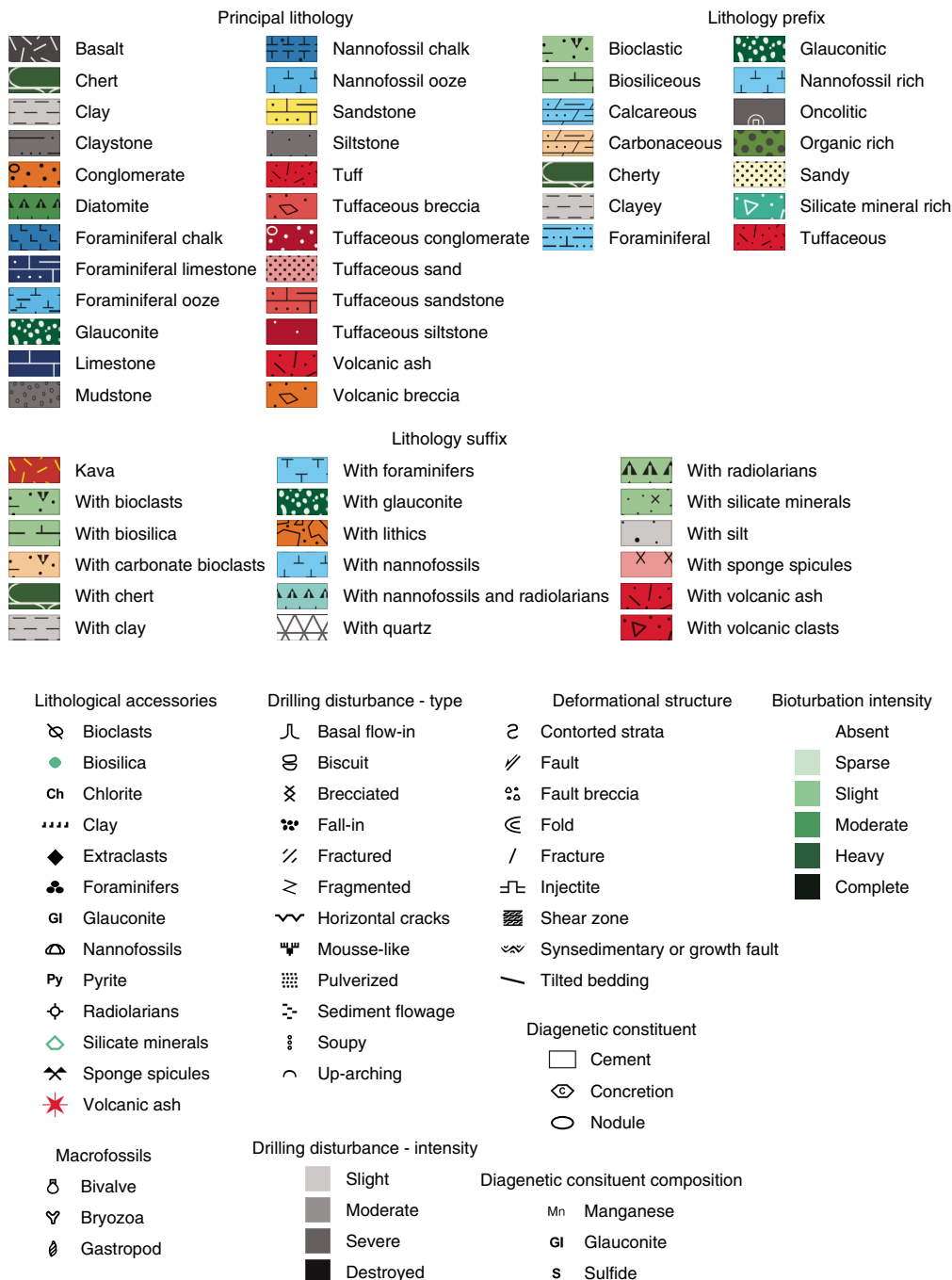
Figure F5. Symbols used on visual core description sheets, graphic logs, and hole summaries, Expedition 371.
