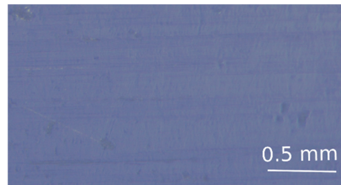
Figure 1. Stereomicroscope image of untreated aluminum surface.
