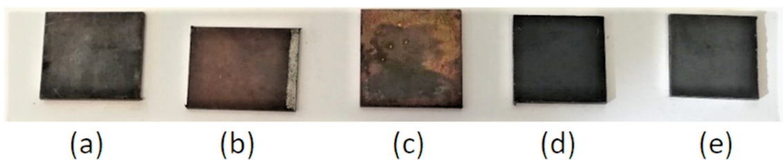
Figure 3. Image of samples treated with solution 1 with different immersion times: (a) 15 min, (b) 30 min, (c) 50 min, (d) 75 min, (e) 90 min.
