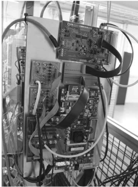
Fig. 6 FPGA board with its signal interface boards
