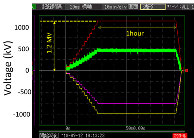
Figure 13. MITICA high-voltage test, first step: 1200 kV for 1 h.
