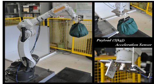
Fig. 21. Experimental system of industrial robot arm
