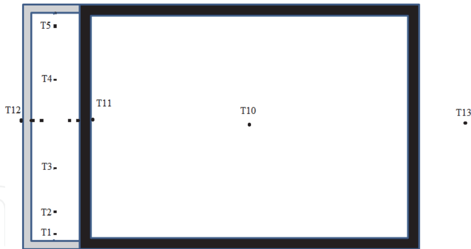
Figure 4. The position of the 13 thermocouples inside the test cell.
