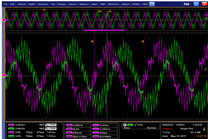
Fig. 8. Phase currents measured with an oscilloscope at the maximum speed of 240krpm. The electrical frequency of 4kHz, corresponds to one tenth of the PWM switching frequency, which is manifested in a distorted phase current.
