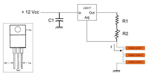
R1 = 6.8  $\Omega$  (0.33 W), R2 = 10  $\Omega$  variable (0.33 W), C1 = 0.1  $\mu$ F ceramic disk or 1  $\mu$ F solid tantalum
