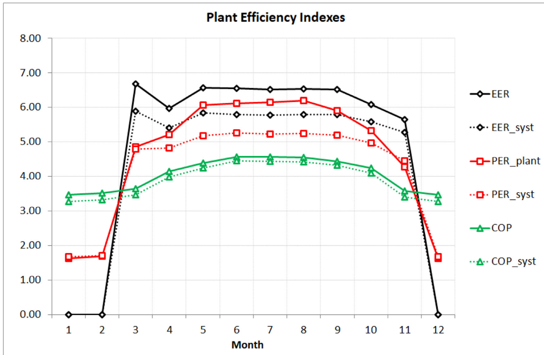
Fig. 14. Heat pump efficiency indexes with pumps parasitic energy (subscript _{\text{syst}} ) or without. PER of the whole plant is represented as well (subscript _{\text{plant}} ).
