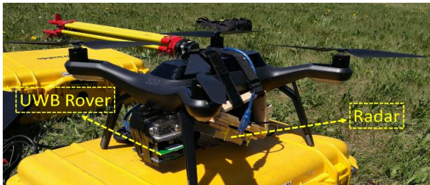
Figure: 3dr Solo quadcopter equipped with micro radar and UWB rover
