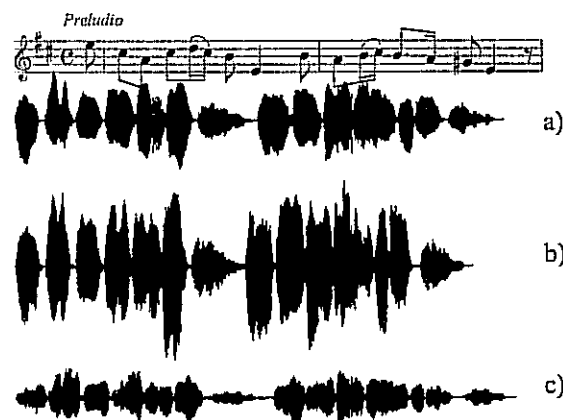
Fig. 3 Violin original: neutral performance a). Violin obtained through post-processing, using time-frequency techniques, from the neutral performance: hard performance b); soft performance c).
