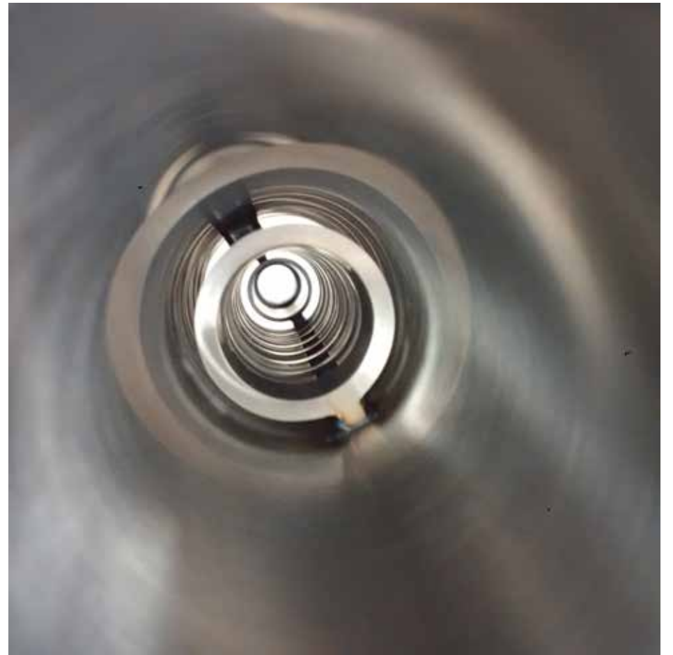
Figure 5. Photograph of the interior of the precision-manufactured MSWS for hot test experiments.
