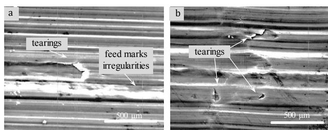
Figure 6. Examples of surface defects found after: a) CT and b) UVT.
