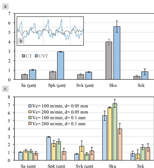
Figure 5. a) Surface texture parameters of CT and UVT; b) 2D profiles; c) surface texture parameters as a function of the cutting parameters in case of UVT.
