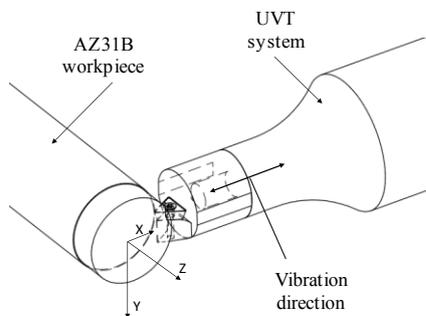
Figure 3. UVT vibration axis along X axis, feed along Z axis.
