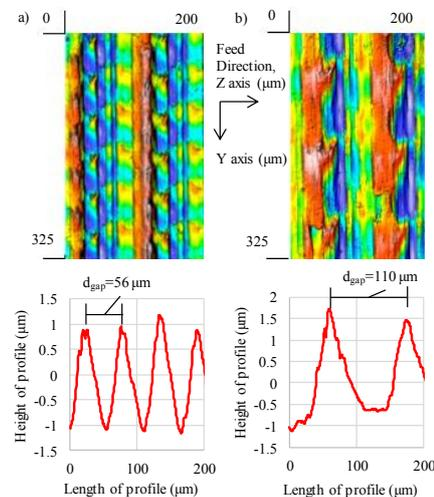
Figure 4. Topography and profile along the Y axis of two samples machined at: a) 100 m/min,  $DOC$  0.1 mm, and b) 200 m/min,  $DOC$  0.1 mm using the UVT system.
