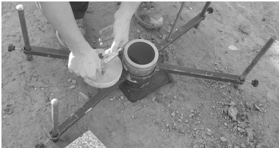
191 192 193 Figure 10. Boutwell permeameter
