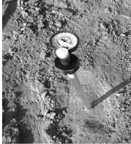
Figure 13. Tensiometers installed on site
