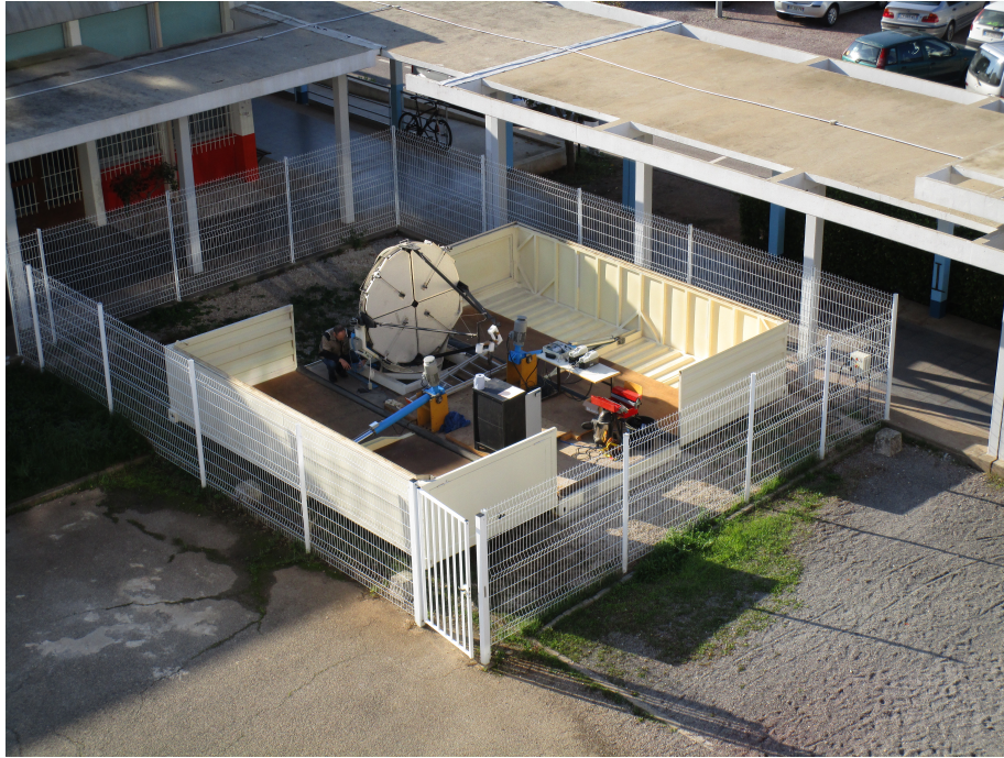
Figure 1: The refurbished CLUE container and UV coated mirror used for the LUPM and IFAE/UAB Raman ILIDARS.
