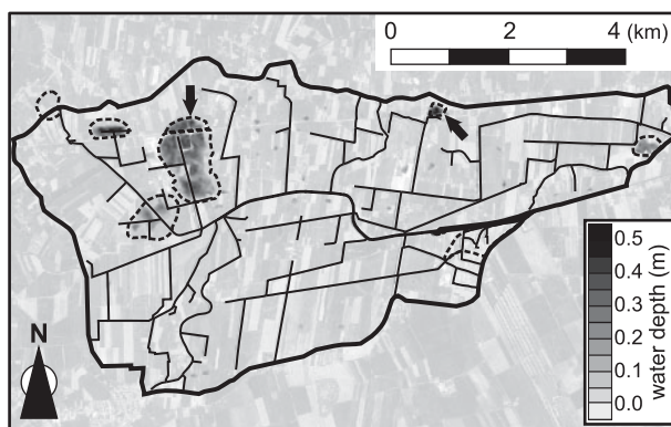
Figure 5. The Rebosola case study. Surveyed (black dashed line) and simulated (gray scale) flooded areas during the storm event of November 2005. Black arrows indicate the areas that are flooded because of inefficiency of the minor drainage network composed of the smaller ditches.
