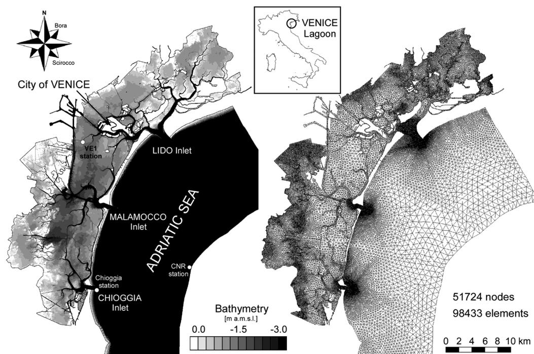
**Figure 1.** Color coded bathymetry of the Venice lagoon and computational grid used for the numerical simulations. The locations of the stations where boundary conditions (Chioggia and CNR-station) are collected and where numerical results are locally analyzed (VE1 station) are also shown.
