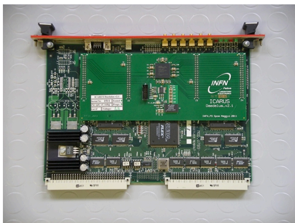
Figure 10. Picture of the ICARUS digital read-out board (CAEN-V789) hosting the S-Daedalus piggyback board.
