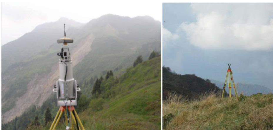
Figure 5. (Left) The Riegl LMS-Z620 with the mounted Nikon D90 digital camera and the Topcon Hiper Pro GNSS receiver on top. (Right) The retro-reflective target used for the back-sight orientation of the scan position.
