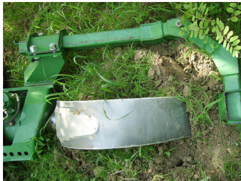
Fig. 1. The semicircular blade and frame of a root-balling machine
