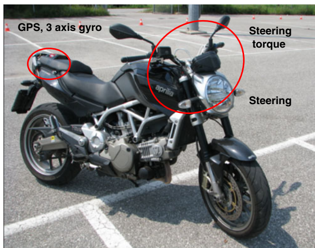
Fig. 6 The UNIPD instrumented motorcycle
