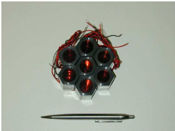
Fig. 1. Prototypes of hybrid photomultiplier tubes.
