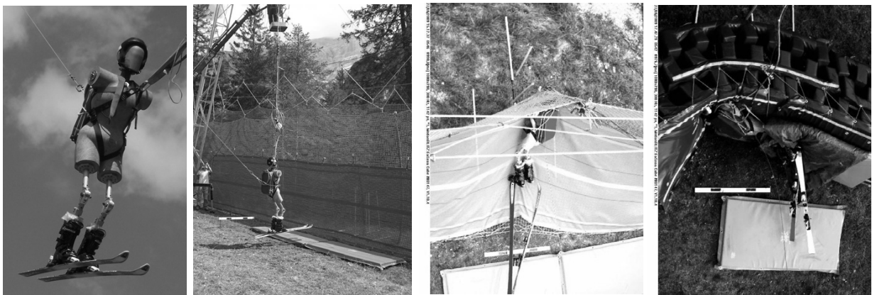
Fig. 5. Field testing with Dummy A1. (a) The dummy A1 during the lifting before impact. (b) The arrangement for testing type A nets. (c) Maximum penetration instant for dummy A1 against type A net. (d) Maximum penetration instant for dummy A1 against foam mattress.
