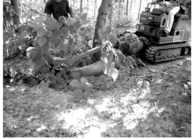
Fig. 1 - A Holmac root-balling machine: in the foreground is a semicircular blade.
