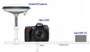
Figure 5: Phisical arrangement of Backpack components.
