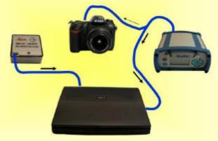
Figure 4: Connections between Backpack MMS components.
