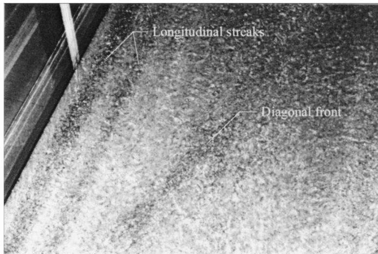
Figure 4. An example of the bed texture observed in run P0109 showing the coexistence of longitudinal alternate streaks of coarse and fine material and diagonal fronts of coarse particles associated to the incipient growth of alternate bars.
