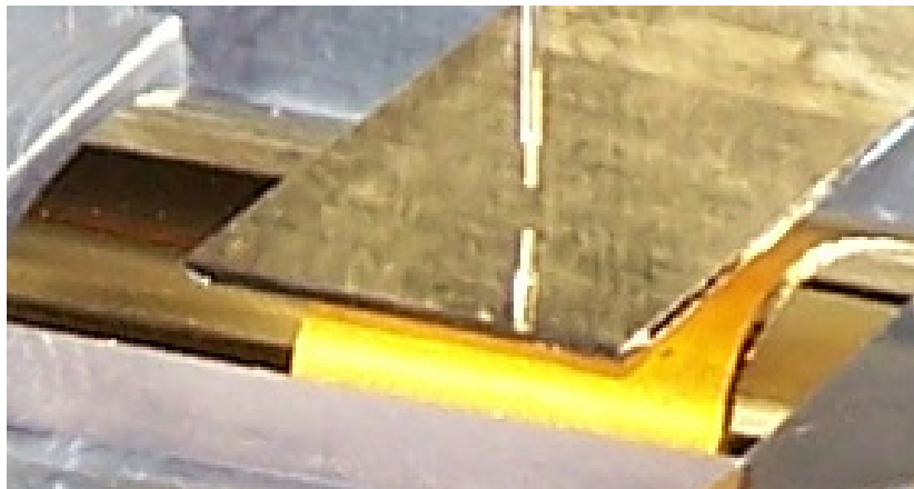
Figure 4. Image of the experimental set-up for the study of the cylinder-plane configuration, with (from top to bottom) the optical fibre for the displacement measurement, the silicon rectangular cantilever, and the cylindrical lens. Cantilever and cylindrical lens, coated with (144 \pm 20) nm of Au, have respectively width and radius of curvature equal to 1 cm. Notice the mirror image of the optical fibre on the cantilever, which allows to estimate the fibre to cantilever distance. With proper illumination and the use of an optical microscope by looking at the mirror image of the cylinder on the cantilever, it is likewise possible to estimate the cylinder–cantilever distance at large (above \simeq 10 \mu\text{m} ) gaps, which allows for consistency checks with the electrostatic calibrations.
