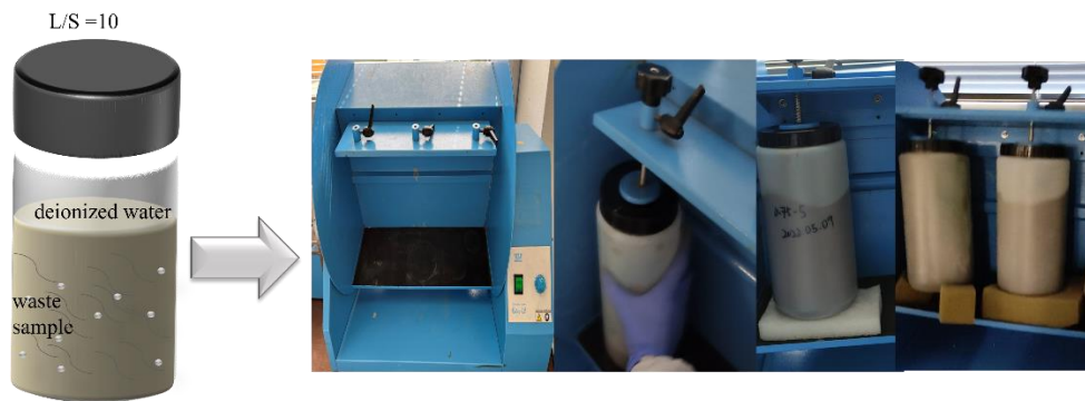
Figure appx. 2. Apparatus for standard batch leaching test (UNI EN 12547-2: L/S=10, duration 24 h)
