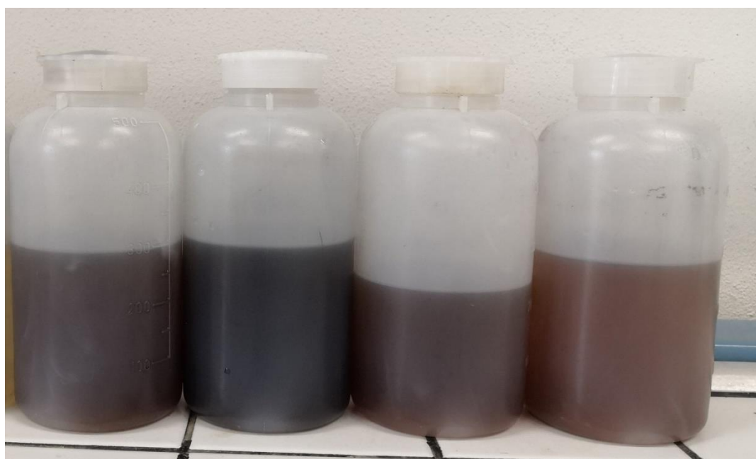
Figure appx. 8. Leachates collected from column tests carried out on old-age residues.
