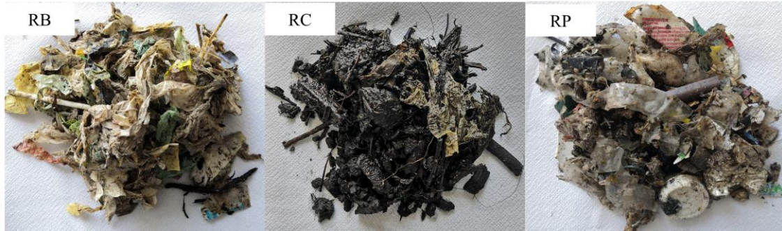
Figure 3.2. 2. The tested raw residues (RB: oversieved residues from separately collected bio-waste; RC: oversieved organic waste after composting; RP: oversieved plastic materials from mixed waste treatment).
