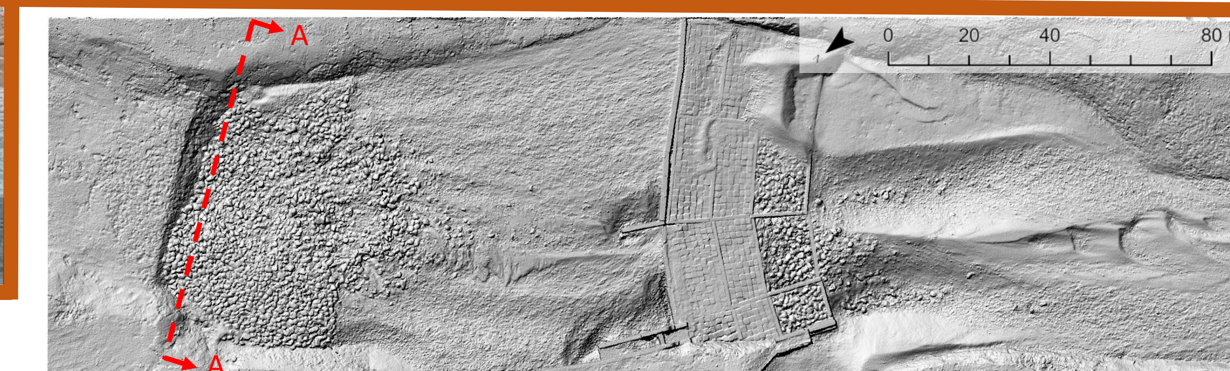
Fig. 3.3: effects of the Q = 714 \text{ m}^3/\text{s} with the designed riverbed protection
