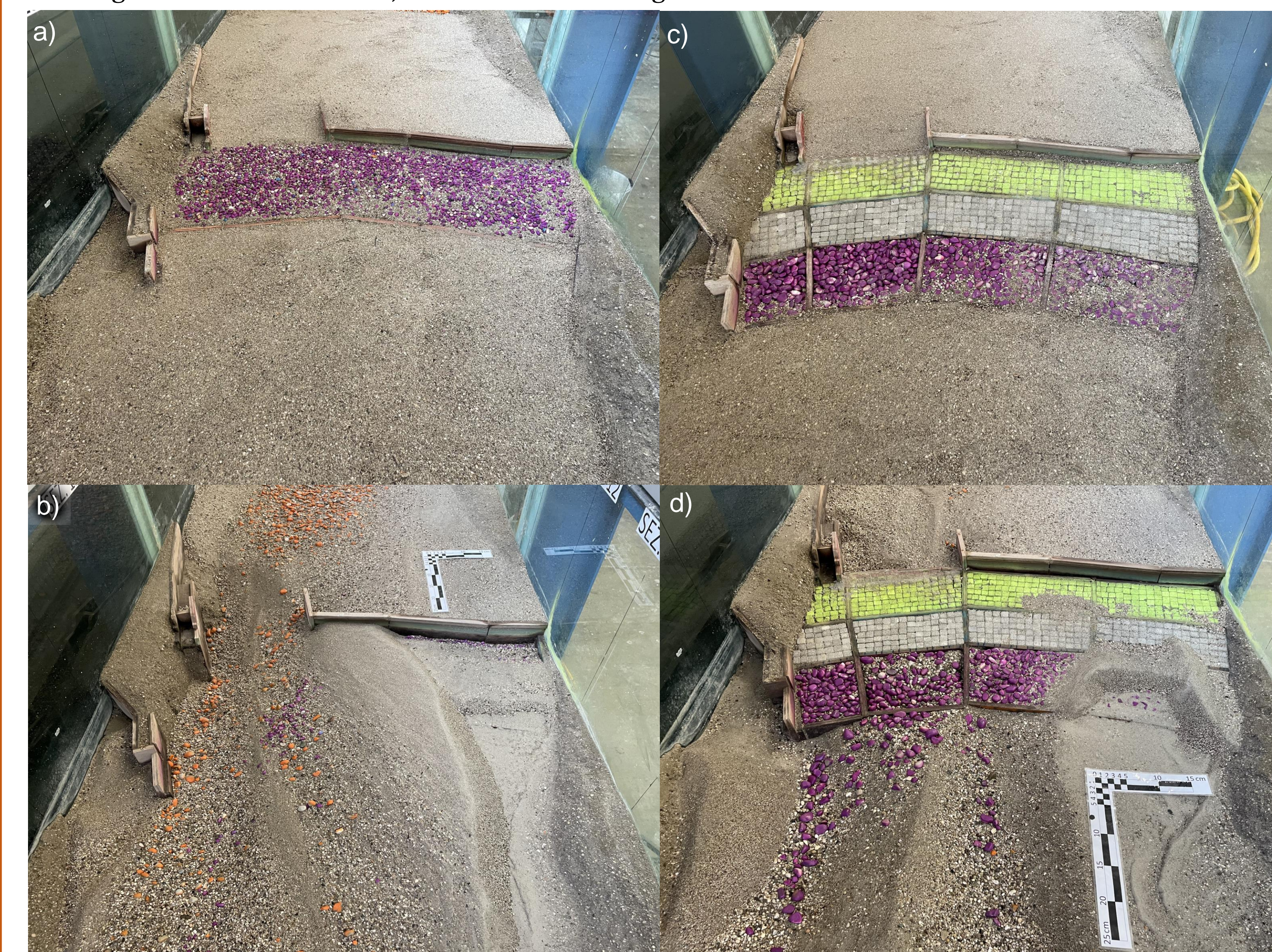
Fig. 2.1: original riverbed protection a) before and b) after the experiments and designed riverbed protection c) before and d) after the experiments
