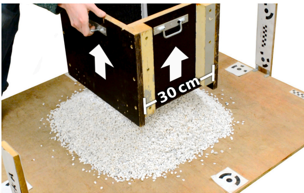
Fig. 4. Dynamic AOR estimation by slowly lifting a wooden mold filled with sediment. The same 30 \times 30 \text{ cm} mold was used as for creating the initial frozen blocks of sediment but with a removed bottom plate. The mold was lifted at roughly 2 \text{ cm per second} .
