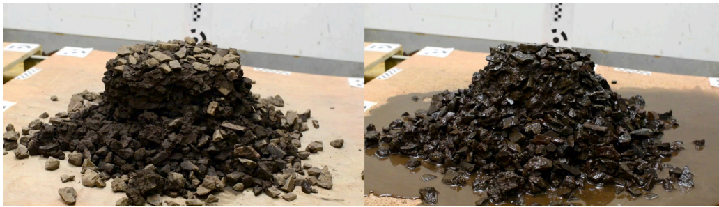
Fig. B.4. Photographs of block of initially ice-cemented sediment (left) after 48 h after degradation and (right) after 60 s of simulated precipitation by a watering can. The sediment was obtained from field molard material from the Árnesfjall landslide (Morino et al., 2019).
