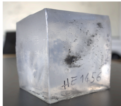
Fig. 6. Soft ballistic gel catcher placed behind the target.
