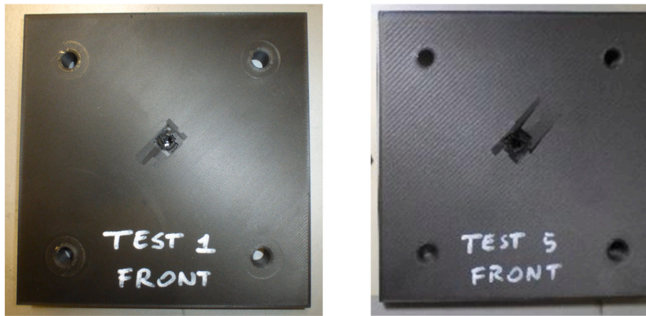
Fig. 7. Test 1 and Test 5 after impact. For the samples printed “horizontally” damage is localized and delamination of the first layers has been detected.
