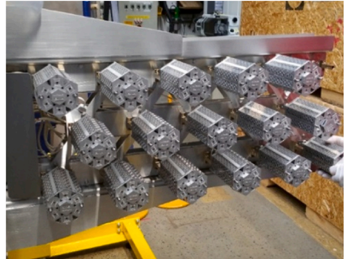
Fig. 10. Picture of mockup pump fully assembled with 17 cartridges.
