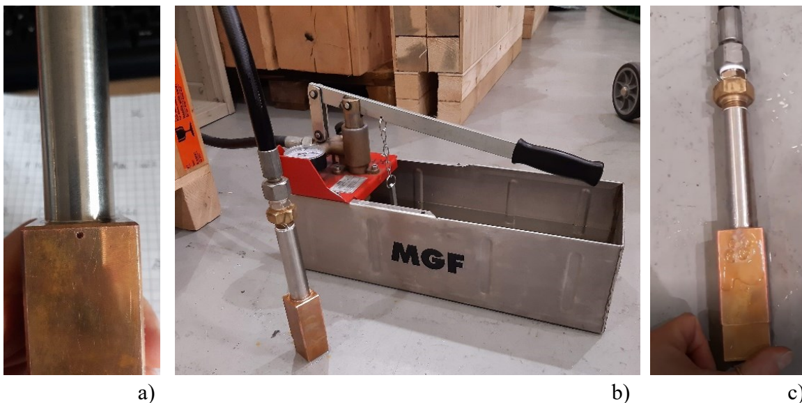
Figure 5.7: a) Hole made on VTTJ Cu side to detect water stagnation area; b) Test set up; c) Water leak from the hole
