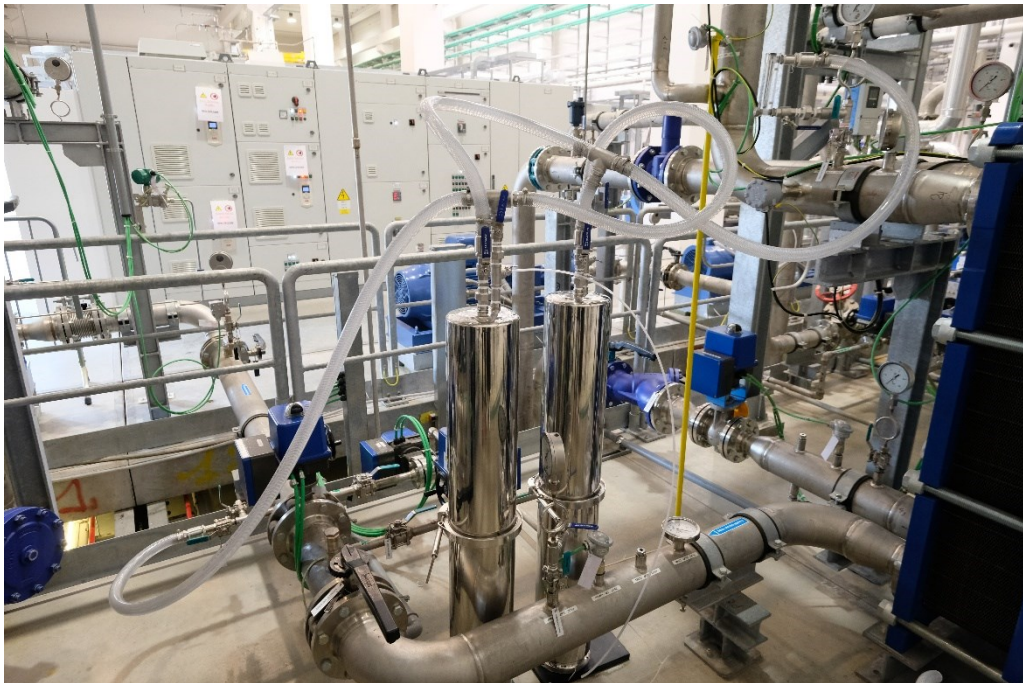
Figure 7.10: a) PC08 scheme when water circulation tests were performed. “R1” and “R2” stands for resin n.1 and resin n.2, b) image of the resins installed in PC08
