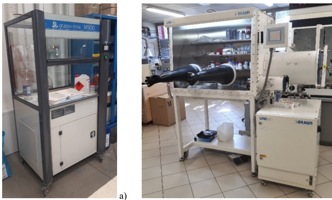
Figure 5.8: The working environments in which the experiments were conducted (a) M900 chemical hood at NBTf used for experiments in HO, providing a controlled oxygen atmosphere.(b) UNIlab LMF Glove Box from the ICMATE Institute used for experiments in LO, enabling work in a controlled oxygen environment.
