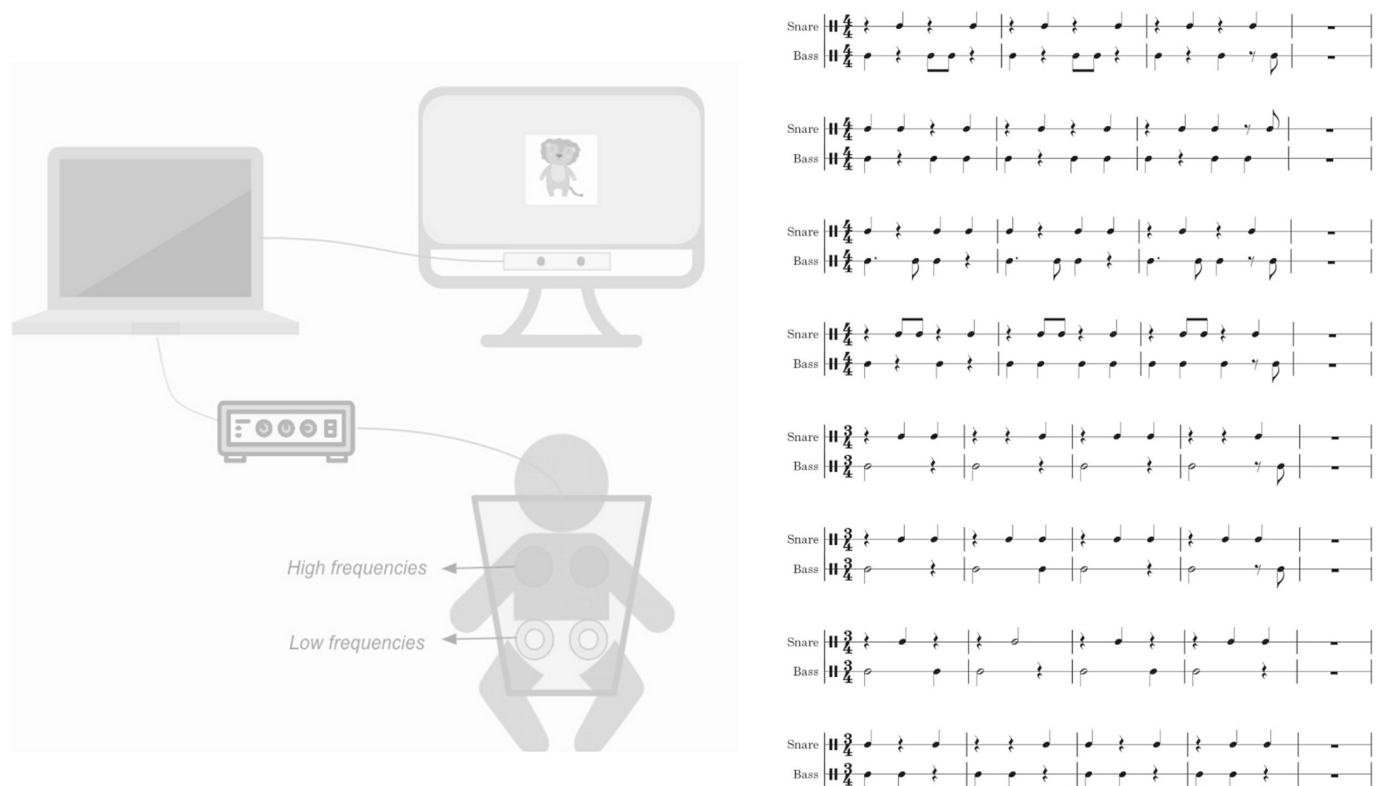
Fig. 2. The Infant vibrotactile system and the displayed rhythms. The experimental set-up included: the laptop running the experiment, the monitor displaying the visual stimuli, the eye-tracker collecting data, the amplifier, and the Infant Vibrotactile System transmitting VTS stimuli in low and high frequencies through actuator channels to the upper and low part of the infant's seat-back.
