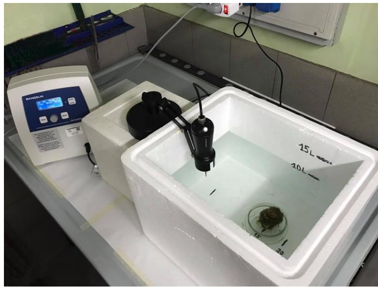
Figure 4. A visual representation of the ultrasound tank set up. The walls of the tank were composed of polystyrene (40 mm in thickness). The tank was filled with 10 L seawater. Externally, mobile support allowed for the tip of the device to be held in place. The tank housed an ascidian individual placed in a glass beaker at 150 mm from the tip of the device.
