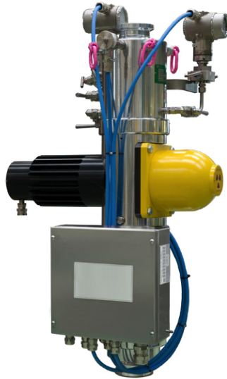
Figure 1. Example of a modular topside Multiphase Flow Meter (MPFM). The vertical pipe is the Venturi tube, where the mixture coming from the well flows. The horizontal tube is the densitometer, while the pressure, impedance and temperature probes are hidden inside the pipe.
