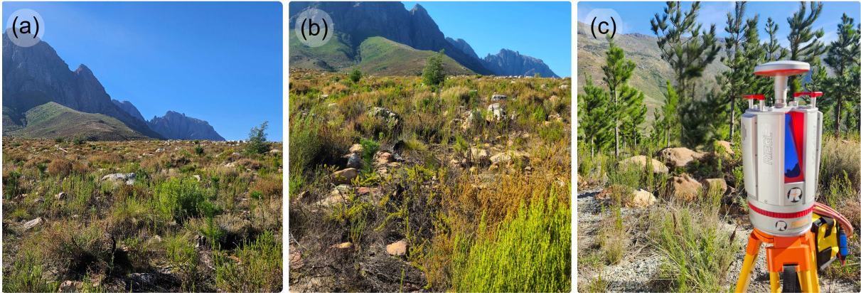
Figure 4.2: Overview of the study area located in a post-fire pine plantation landscape in the Jonkershoek Nature Reserve, Western Cape, South Africa. (a–b) Typical terrain and vegetation conditions during data collection, showing exposed rocks and dense low-vegetation regeneration. (c) The RIEGL VZ-2000i terrestrial laser scanner used in this study.
