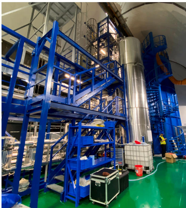
Fig. 6. Stripping plant installed in the Underground LS Hall at the JUNO site.
