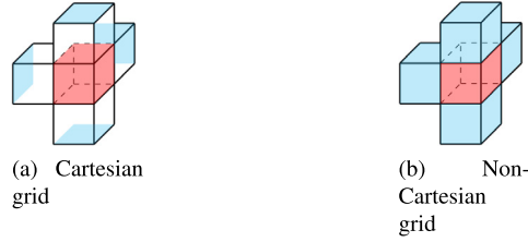
Fig. 3. Sketch of the base patterns for Cartesian and non-Cartesian grids. The front and right elements have been removed to improve the readability of the subpanels.
