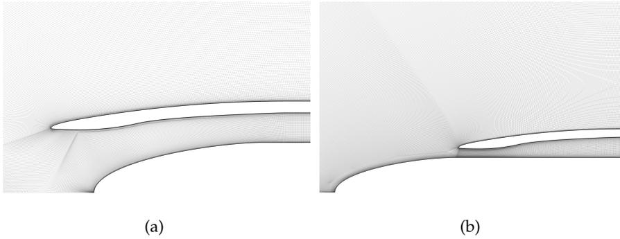
Figure 3.3: Closeup view of the computational grid around the intake wall for both fully-retracted (a) and fully-extended (b) configuration.
