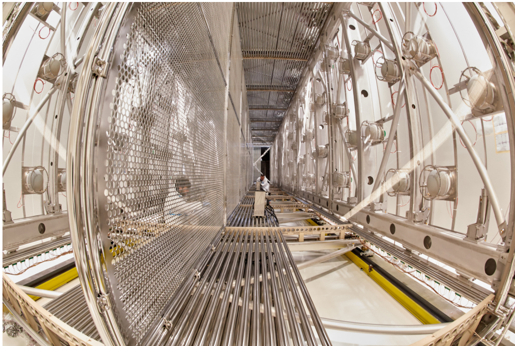
Figure 3.13: Inner view of one ICARUS module with the two TPCs separated by the common central cathode and showing the new 8" PMT system behind the wire planes. Figure courtesy of CERN, where the picture was taken during the refurbishing in a clean room.
