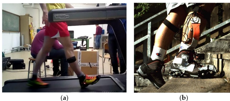
Figure 3. Data collection sessions: (a) example of data collection of one subject wearing TR shoes, walking at 5 km/h on a treadmill with an inclination of 5%; (b) example of data collection of one subject wearing CH shoes climbing a flight of stairs outdoor. Both IMU and video based acquisition systems were used together.
