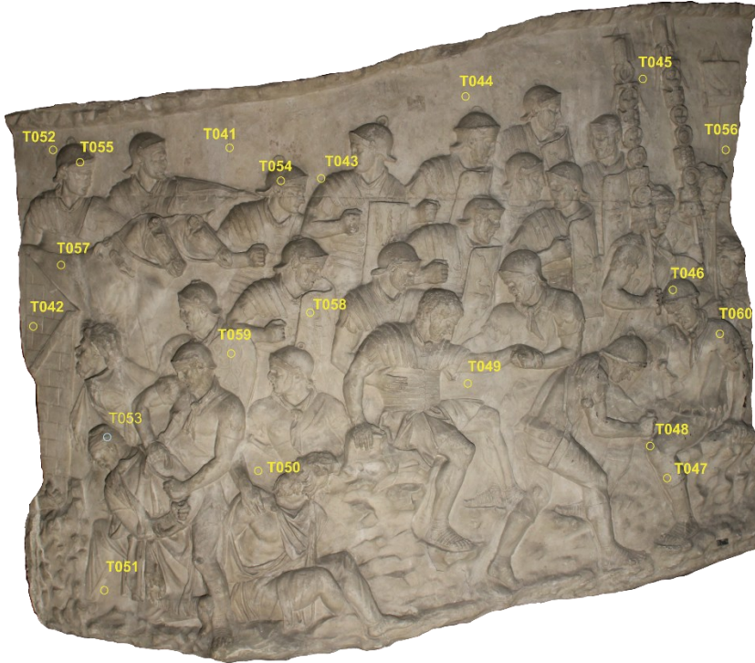
Figure 15. Colourimetric measurement points (T_041 to T_060) on the surface of plaster replica MCR_3052, acquired in the CIELab* colour space. The distribution of points was designed to sample areas with varying surface conditions to assess chromatic alterations.
