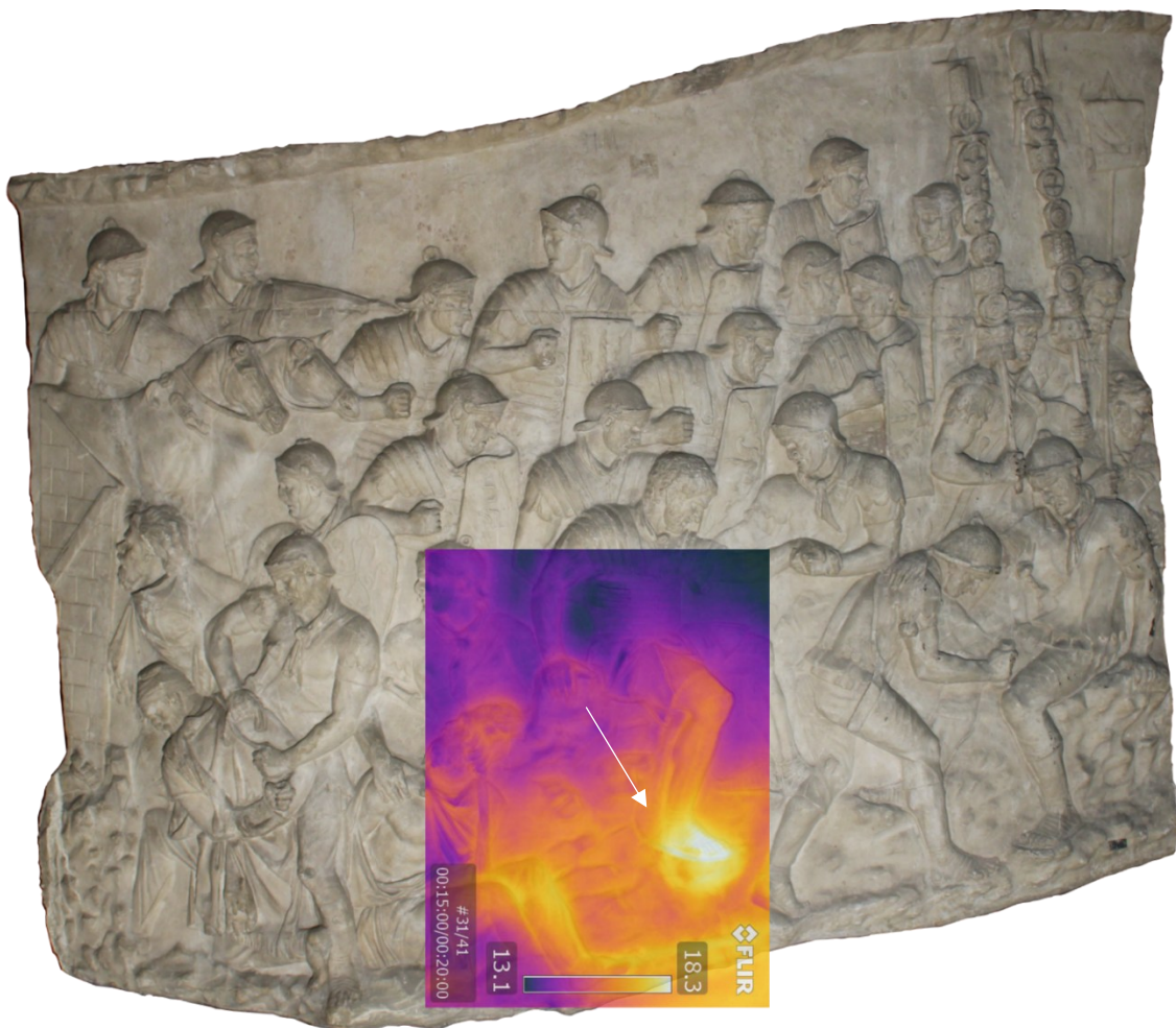
Figure 16. Overlay of the plaster replica MCR_3052 with the active infrared thermographic acquisition. The thermogram, obtained during a time-lapse cooling phase, reveals thermal patterns in the central area of the cast. The vertical zone with higher thermal response (yellow-orange tones) corresponds to a known fracture, as indicated by the white arrow, while other variations in thermal behaviour may indicate material inconsistencies or prior restorations not visible in standard imagery.
