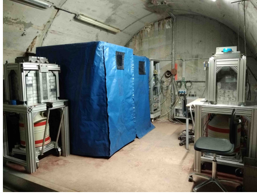
Figure 4.4: Measurement platform in the HADES underground laboratory. The static tables with the lead castle are visible.
