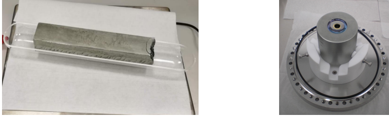
Figure 4.2: Left: starting material, Ge metal ingot. Right: final product, example of Coax detector.
