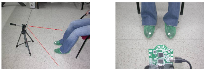
Fig. 1. In the left image, the relative position of the user and the infra-red camera can be observed. The right image shows a view of the reflective markers from the camera perspective.
