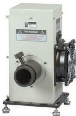
FIGURE 4.17: Low cost solar simulator. It implies a 150W Xenon lamp to reproduce the sunlight spectrum.
