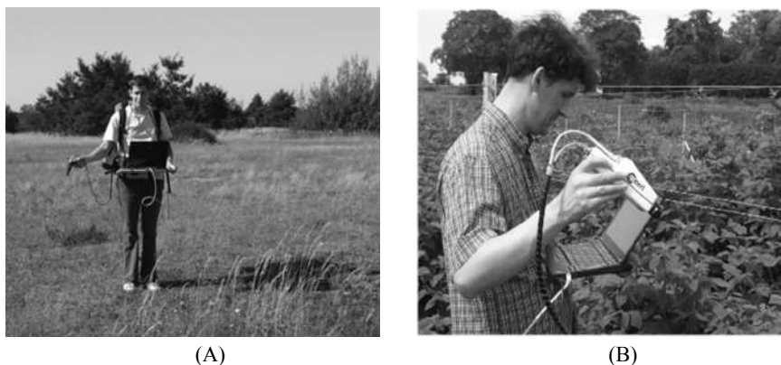
Fig. 1: A non-imaging (A) and an imaging spectrometer (B) in field use ( Source: A. Jung)
