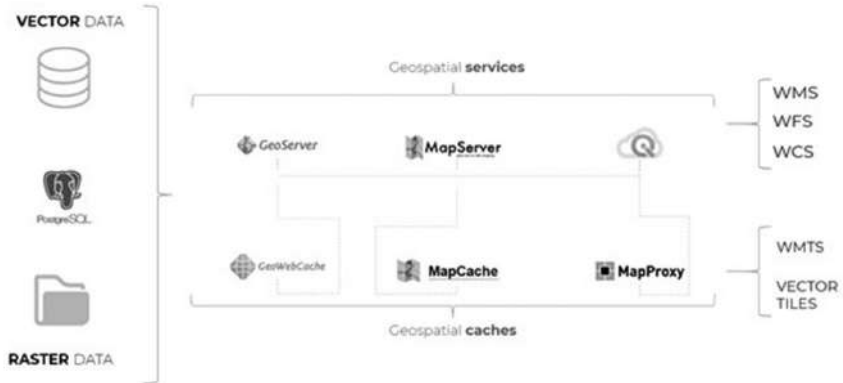
Fig. 4: Examples of software products to set-up the back-end architecture of a web mapping application ( Source: Authors' elaboration)
