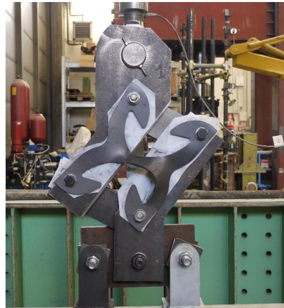
Fig. 25. Deformed specimen in shear
