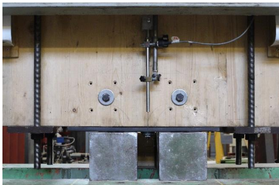
Fig. 10. Anchoring of concealed X-bracket type 2 to CLT with special elements without the use of complementary plates or additional fasteners (panel-to-foundation joint)
