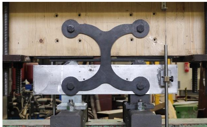
Fig. 5. Alternative usage of the X-bracket type 2 as external connection
