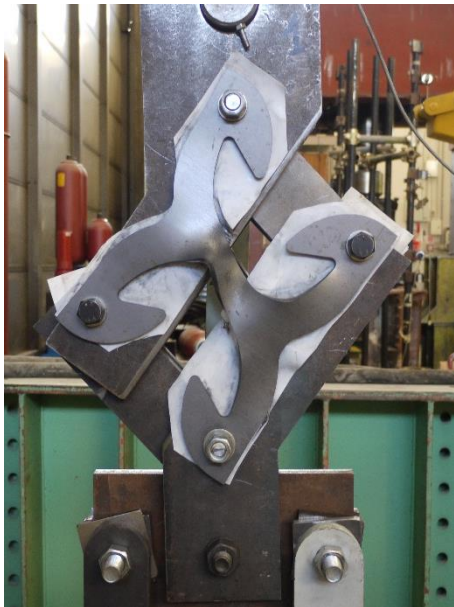
Fig. 24. Deformed specimen in tension: (a) Loading; (b) Unloading
