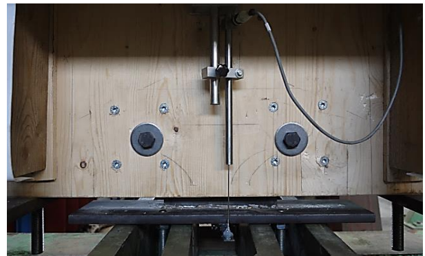
Fig. 9. Anchoring of concealed X-bracket type 2 to CLT with self-drilling dowels (panel-to-foundation joint)
