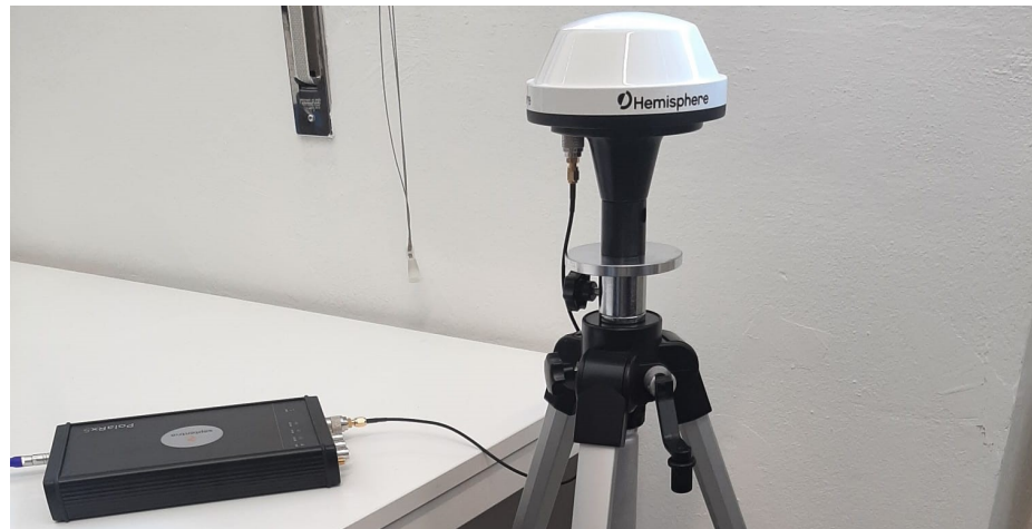
Figure 4. Setup used for the experimental dataset collection: Septentrio PolarRx5 receiver connected to an A42 Hemisphere antenna.
