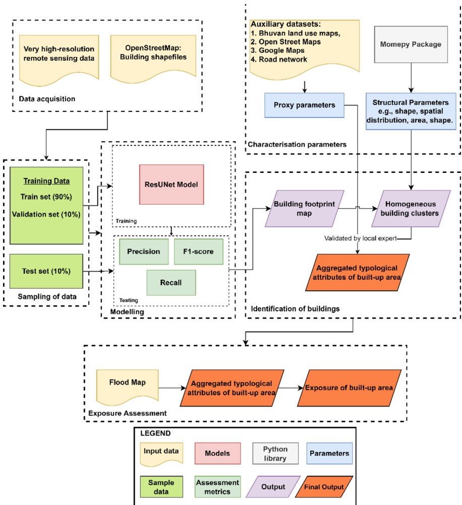
Fig. 2 Conceptualisation of the research methodology. The steps include the preparation of data, sampling of the data for model training and evaluation, calculation of characteristic parameters combining these parameters into typological attributes of the buildings at an aggregated scale, and exposure assessment of the aggregated buildings using the derived typological attributes
